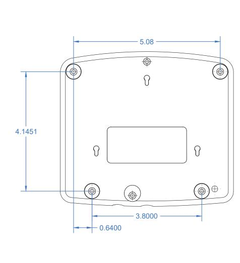
Screw is 4-20 x 0.25 thread forming screw
